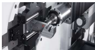
タッピング装置 Integration of an additional machining process
